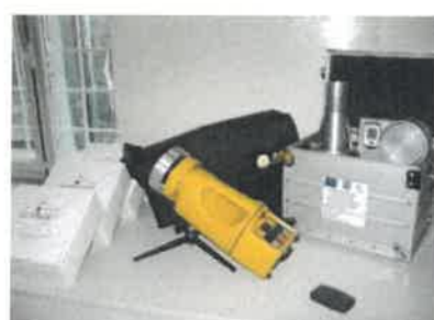
Prelevator SAS aeromicroflora
