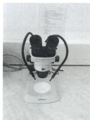
Binocular stereomicroscop SZ51 / Olympus
