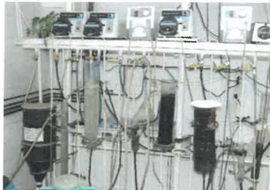
Instalatie biologica in flux continuu
