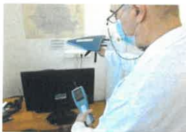
Sistem de monitorizare camp electromagnetic
